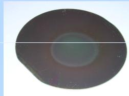
Sol-gel derived PZT on 2 inch NCD-on-silicon wafer
