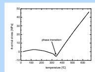
calculated thermal mismatch of PZT to substrate after deposition
