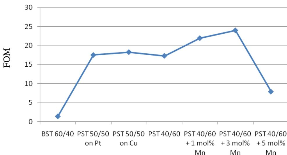
Fig. 1: The figure of merit of different ferroelectric perovskite thin films presented in the thesis.
