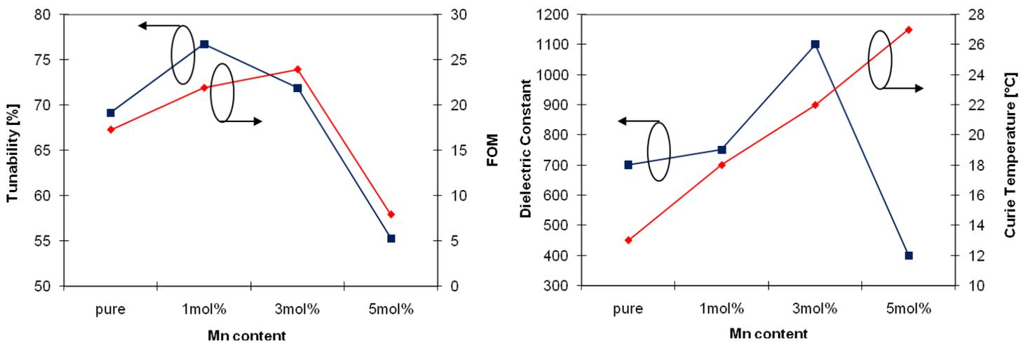
Fig. 2: Tunability and figure of merit at 10V and dielectric constant and Curie temperature at zero bias of PST 40/60 with different Mn content
